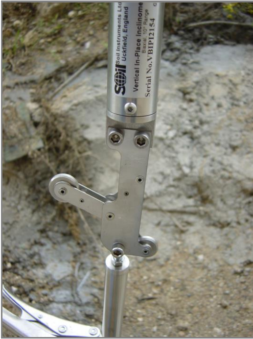
Above: Detail of gauge rod/wheel/sensor body built up prior to installation
