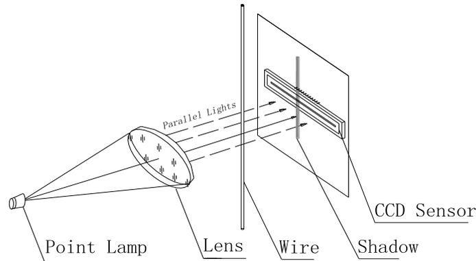
The illustration of the principle of CCD imaging
