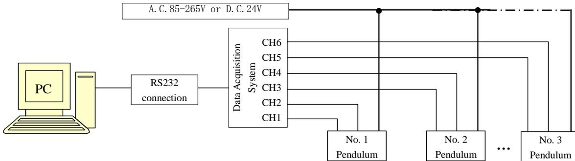
Measuring analogue signals using a Data Acquisition System
