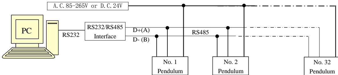
RS-485 network formed by the Automatic Pendulum Systems
