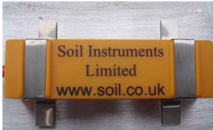
Coil Assembly with securing straps in place prior to welding
