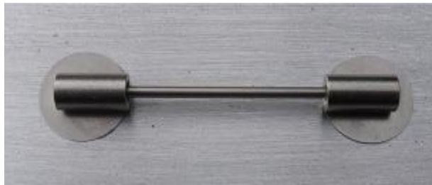
Gauge positioned on cleaned surface ready for installation
