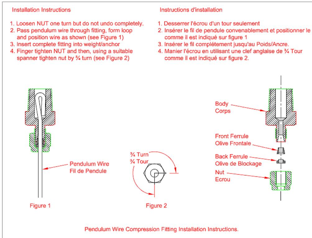
A suitable pull-test should be carried out to ensure that the wire is clamped correctly. Screw the fitting back into the anchor without twisting and kinking the wire then fully tighten.
