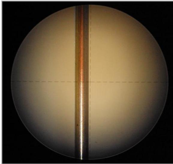
With the graticule aligned with the edge of the wire the microscope position is read-off the vernier scale and recorded.
