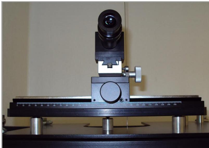
The co-ordinate position of the pendulum wire relative to the fixed reference frame is determined by adjusting the position of the microscope to view the edge of the wire against a graticule on the telescope lens.
